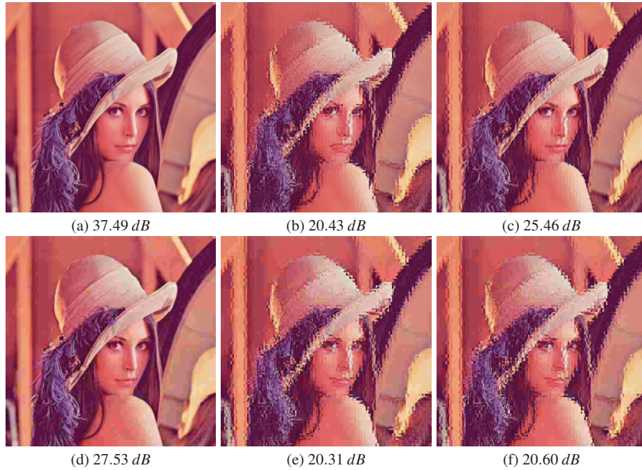
Fig. 7 a) JPEG compressed image with QF=100%, b) Image (a) with C = 128 bits/block, c) Image (a) with C = 8 bits/block, d) JPEG compressed image with QF=10%, e) Image (d) with C = 128 bits/block, f) Image (d) with S = 8 bits/block.
